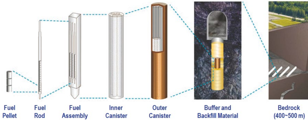
Fig. 1. Schematic diagram for multiple-barrier system incorporated in the KBS-3 type disposal concept.
