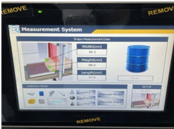
Fig. 9. Shape acquisition of radioactive metal waste samples.
