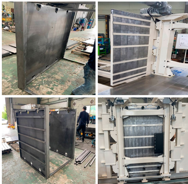
Fig. 4. Lead shielding device assembly design and manufacturing.
