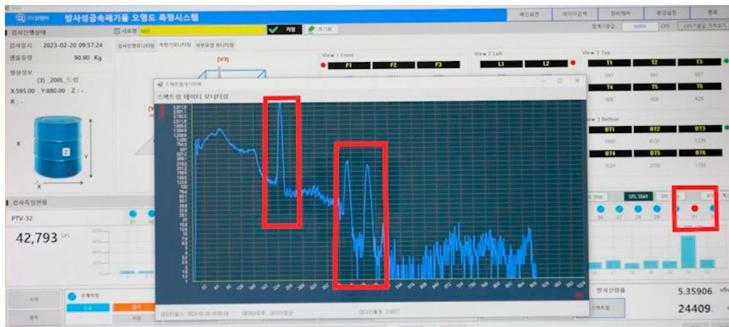
Fig. 12. Gamma-ray measurement using LBC detector ( ^{137}\text{Cs} , ^{60}\text{Co} check source).
