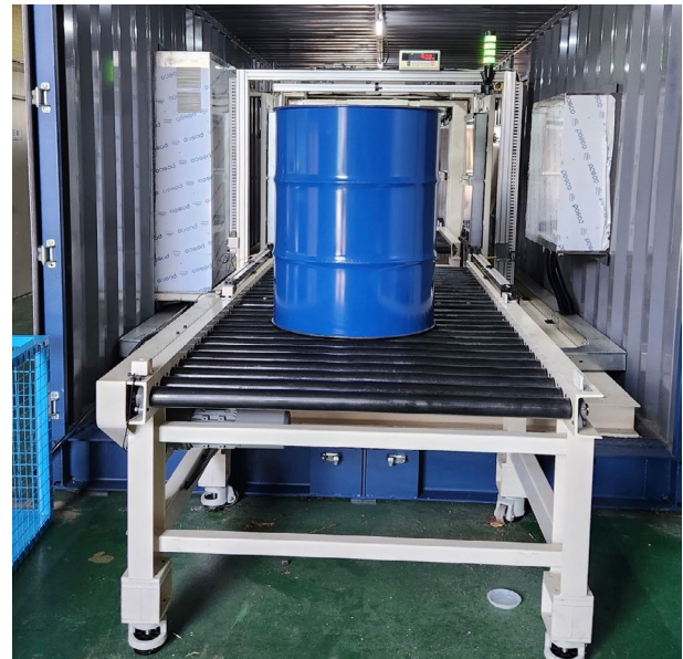
Fig. 8. Radioactive metal waste measurement pilot operation.
