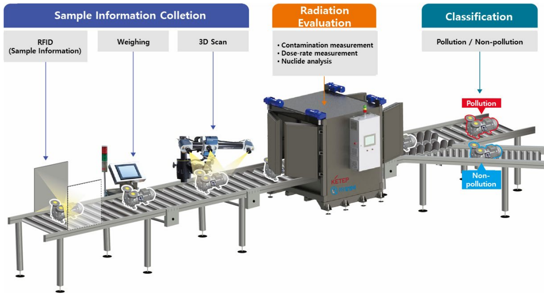
Fig. 1. Metal waste measurement and classification system.
