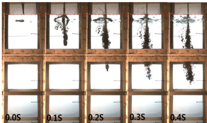
Fig. 6. Jet breakup process of MATE 09 experimental test [20].
