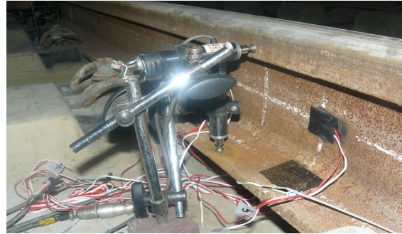
(a) Rail vertical displacement measured
