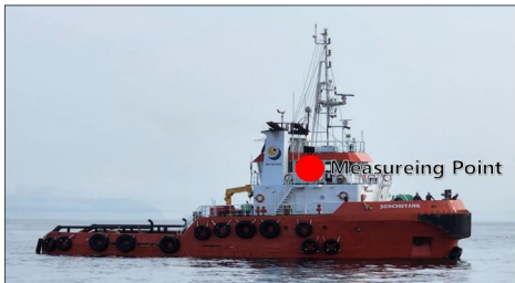
Fig. 4. Installation location of measuring sensor.
