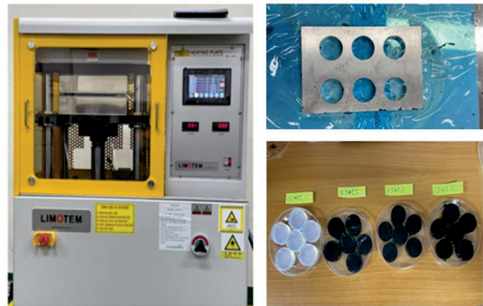
Fig. 2 Automatic heating plate (QM900A), Compression set test specimen
