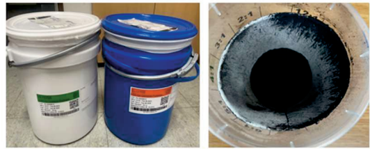
Fig. 1 Liquid silicone rubber (SL 7220), Carbon Black sample (CAS 1333 86 4)
