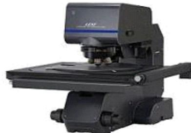
Fig. 4 Equipment for measurement - 3D Laser Confocal Microscope
