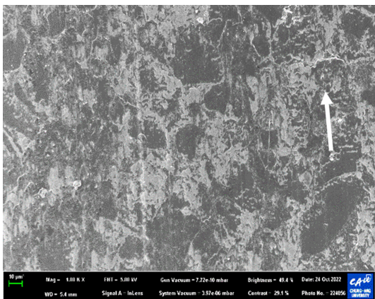
Fig. 7. Wear track of 0.2 vol. % filled PTFE taken at X 1,000. The arrow indicates sliding direction.
