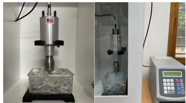
Fig. 3. Photographic images of equipments used for ultrasonic tip sonication process
