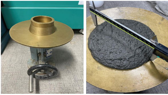
Fig. 6. Example of mortar flow test
