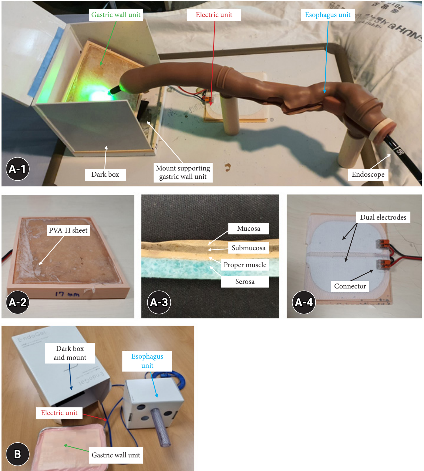
Fig. 1. The new endoscopic submucosal dissection (ESD) simulator is composed of three units: the esophagus, gastric wall, and electric units. (A-1) The esophagus unit aids endoscopic insertion. (A-2) The gastric wall unit is connected to an electric surgical unit. (A-3) The gastric wall unit is designed to have three layers of different types of polyvinyl alcohol hydrogel (PVA-H) sheets. (A-4) An electric surgical unit. (B) An existing ESD simulator is composed of three units.
