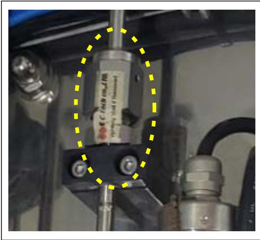
Fig. 7. Attaching a marking label for male and female threads.
