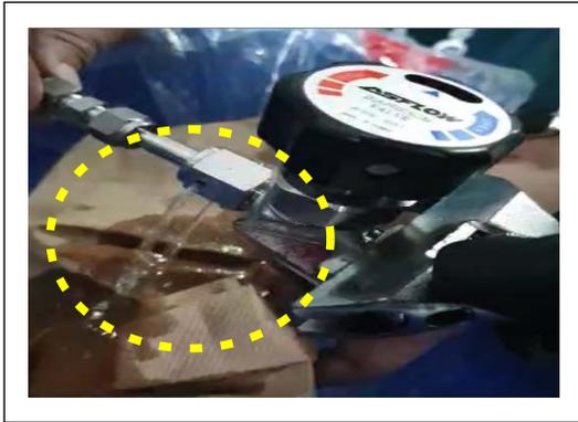
Fig. 4. Simulation in case a thread is released by a 15 degree.
