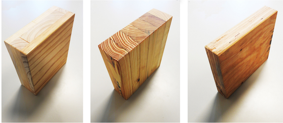
Figure 1. From left to right: Cross Laminated Timber (CLT), Glued Laminated Timber (GLT) and Laminated Veneer Lumber (LVL) (Source: G. Marfella)
