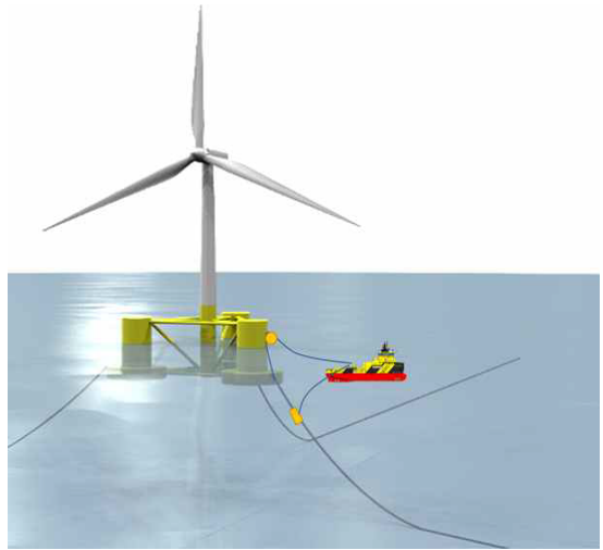
Fig. 1 Concept of disconnectable mooring system for FOWT
