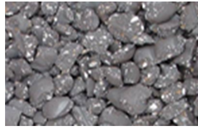
Fig. 10. Briquette produced by adding Anthracite and Binder to the Fe-clinker.
