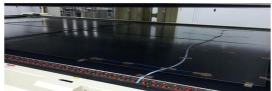
Fig. 3. Laminating equipment with Multi zone silicone rubber heater
