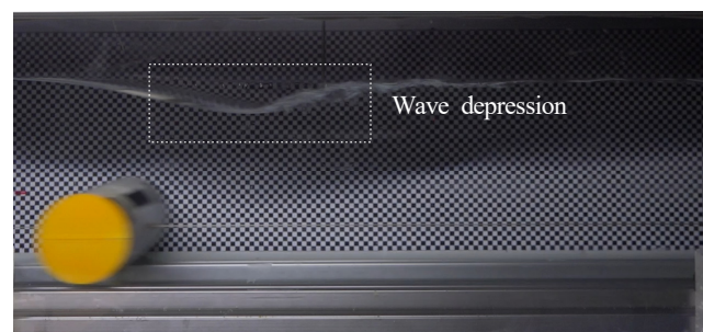
Fig. 1 Free surface wave depression caused by submerged cylinder motion
