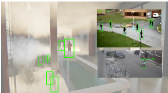
Figure 11. Detection and numericalization of pedestrian in building by mechanical learning
