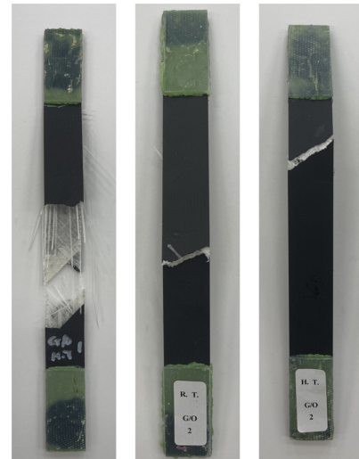
Fig. 7. Failure mode of G.O. (HSHT glass + Onyx)
