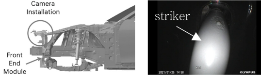
Fig. 7 The Camera Installation on Front End Module and Captured Image of Video Footage in Belgian Road
