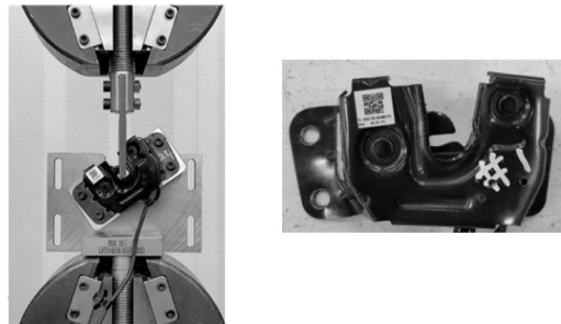
Fig. 17 Test Rig Setup and Test sample for an Oblique Condition
