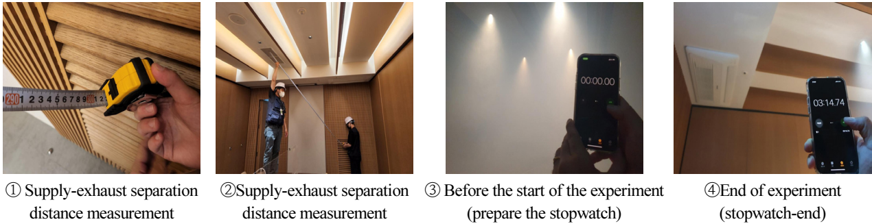
Fig. 9. Test process for interlocking smoke control system in living room of the same area
