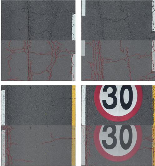
Fig. 14. Comparison of Frame Extraction Images and Crack Detection Results
