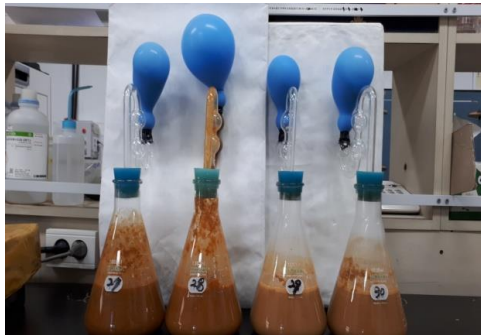
Figure 3: Comparison of the Balloon Volume of Food Wastewater 1, Food Wastewater 1+ Enzyme, Food Wastewater 2, Food Wastewater 2+ Enzyme (from Left)
