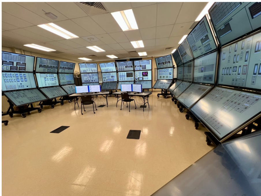
Fig. 4. HSSL after 2022 remodel, featuring adjustable bays with higher resolution and improved touchscreens.
