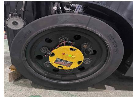
(b) Attached measurement module on forklift's front wheels
