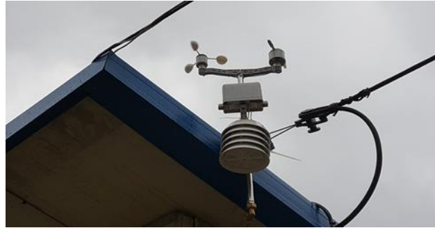
Figure 2. External weather sensor: temperature, humidity, pressure measurement
