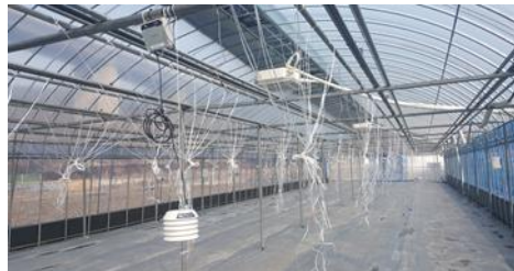
Figure 3. Internal sensors: temperature, humidity measurement
