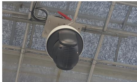
Figure 4. Observation camera: capable of pan, tilt, zoom, and night vision.
