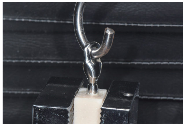
Fig. 3. Universal testing machine (TW-D102; Tae-Won Tech Co., Seoul, Korea) connected to the crown prepared for pull-out test.
