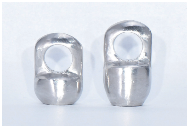
Fig. 2. Laser sintered Co-Cr alloy crowns for 3.0-mm and 6.0-mm abutments.
