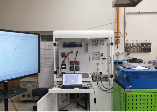
Fig. 2. Evaluation device of water electrolysis cell & stack
