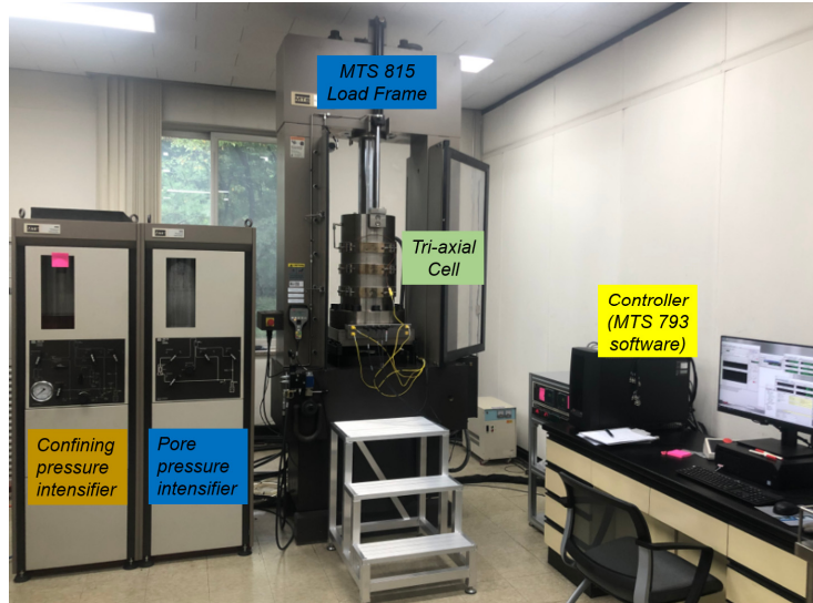
Fig. 3. Triaxial test equipment
