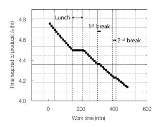
Fig. 3. Short-term learning effect on wet cutting as a function of work time, t.
