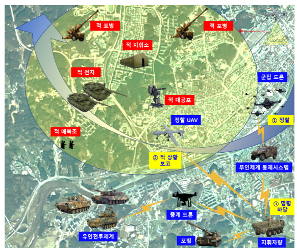
Fig. 1. Expected scenarios for attack drone operation (Phase #1)
