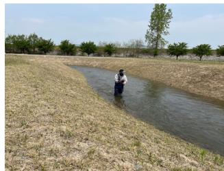
(b) Measurement method of topography using RTK-GPS
