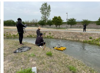
(c) Measurement method of water depth using ADCP
