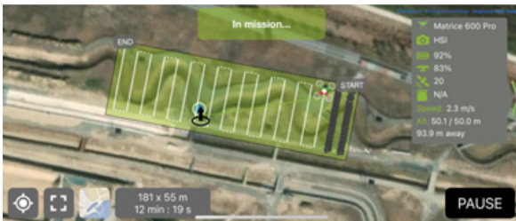
(a) Using RGB image with drone (SfM)
