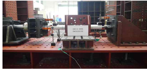
(b) BRB-C Specimen Test Setup
