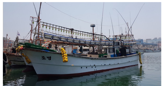
Fig. 1. Induction and metal halide fishing lamp installed fishing boat (Jo-Myeong).
