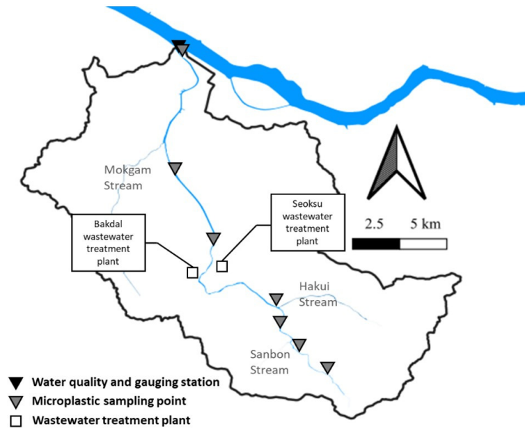
Fig. 1. Anyangcheon stream and its monitoring system for this study. There are two wastewater treatment plants, Bakdal and Seoksu, contributing to the water environment of the Anyangcheon stream
