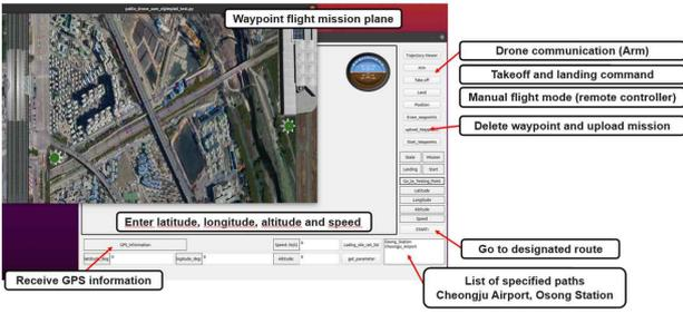
Fig. 13 Flight control system user interface and usage
