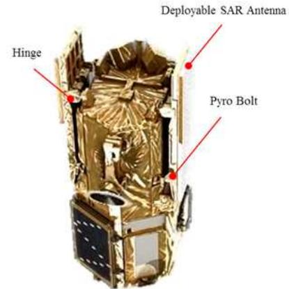
Fig. 1 Example of Deployable SAR Antenna [8]
