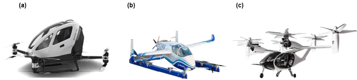
Fig. 1 UAM Aircraft: (a) Multi-copter, (b) Lift+Cruise, (c) Vectored Thrust
