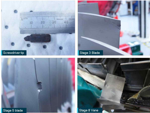
Fig. 1 Screwdriver tip and witness marks [6]
