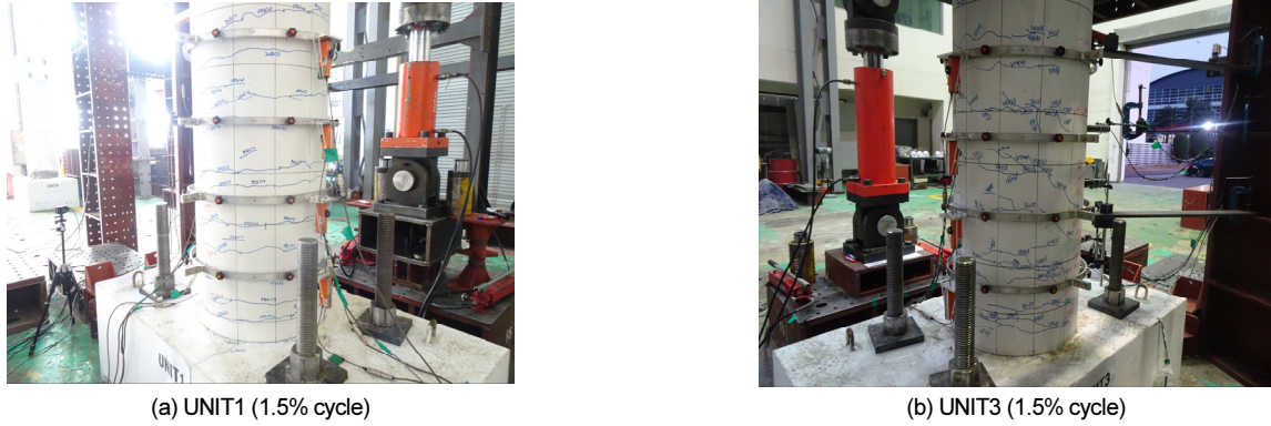
Fig. 4. Representative crack patterns
