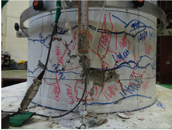
(a) UNIT4 initial spalling at 3%
