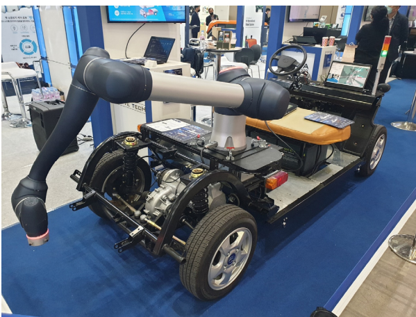
[Fig. 1] Autonomous driving electric vehicle system for logistics with a robotic arm
