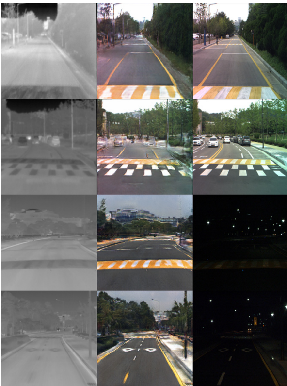
[Fig. 2] Qualitative results of Thermal-to-RGB translation. The first and second rows were taken during the day, and the third and last rows were taken at night. On the left is Thermal, in the middle is Pseudo RGB, and on the right is RGB
