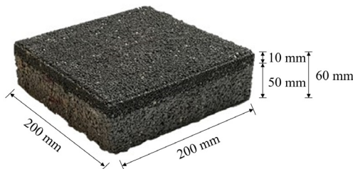
Figure 3. Concrete permeable blocks using real manufacturing procedure
