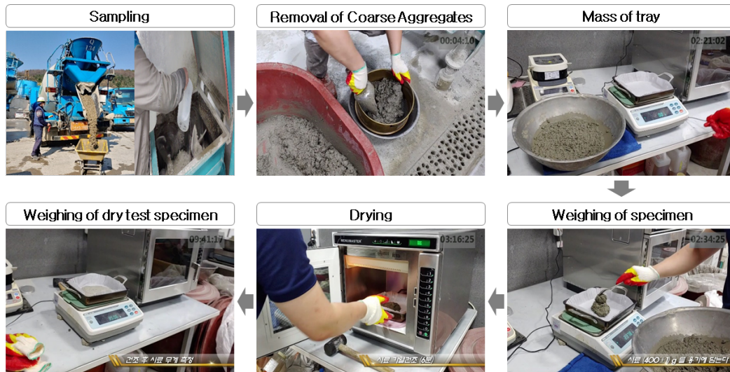
Figure 1. Flow of Microwave Oven Drying Test Method
