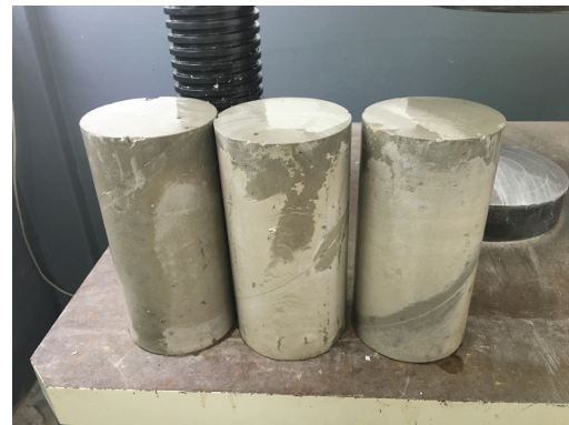
Fig. 1. Cylinder specimen for compressive strength
