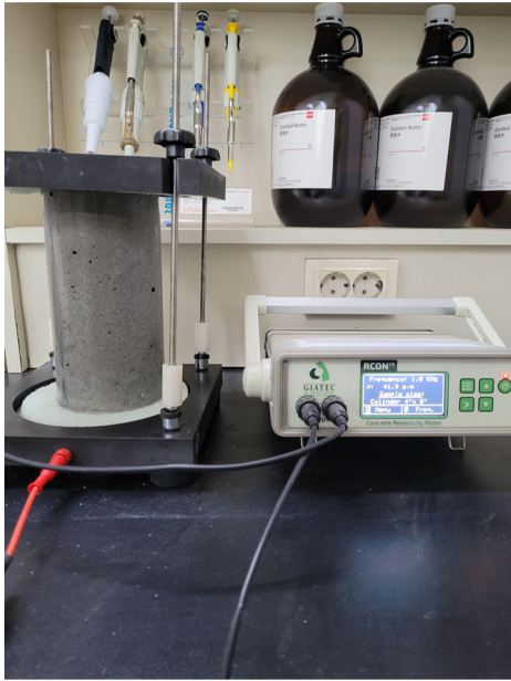
Fig. 8. Non-Destructive Resistivity Measurement Test (RCOM™)
