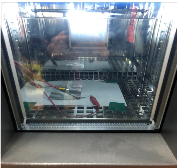
Fig. 3. The experiment of resistance change in a temperature chamber.
