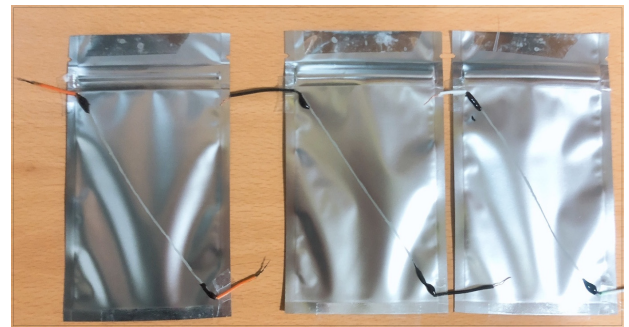
Fig. 1. Aluminum pouch with conductive wire.
