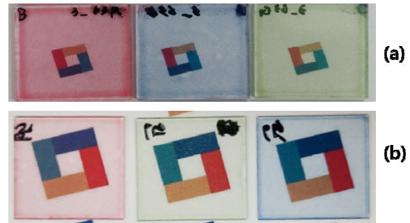
Fig. 6. Photograph of color glass made by (a) NOA 63, (b) NOA 65.
