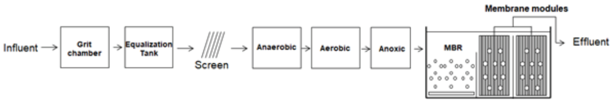
Fig. 1. Schematic of the full-scale wastewater treatment plant.
