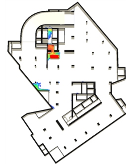
[Figure 2] Distribution of visible distance (After 100s)
