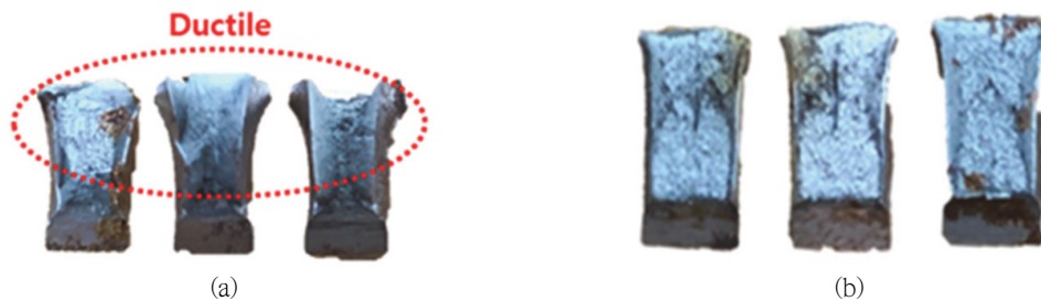
Fig. 3 Temperature-dependent fracture surface for AH36 on the tested temperatures: (a) 20 and (b) -60°C.
